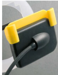
The sensor should be placed as low as possible as shown in this picture. The top edge of the sensor aligns with the midline of the claw.
